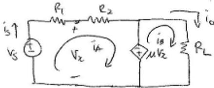
Find an expression for the current gain  $i_B/i_s$  in the circuit
