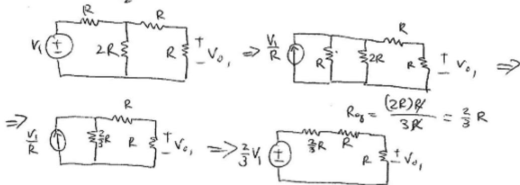
$$\begin{aligned} \therefore V_{o1} &= \frac{R}{\left(\frac{2}{3}R + R + R\right)} \left(\frac{2}{3}V_1\right) \\ &= \frac{3}{8} \left(\frac{2}{3}V_1\right) \\ &= \frac{V_1}{4} \end{aligned}$$
