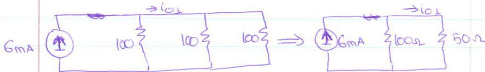
Two path current division  $i_{o1} = \frac{100\Omega}{(100+50)\Omega} \cdot 6\text{mA} = 0.4\text{mA}$
