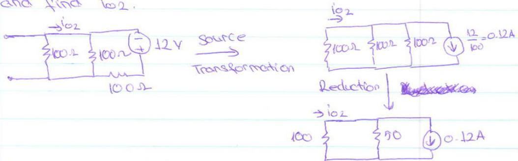
Two path current division  $i_{o2} = \frac{100\Omega}{(100+50)\Omega} \cdot 0.12\text{A} = 0.04\text{A} = 40\text{mA}$
