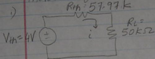
$$i = \frac{V_{th}}{R_{th} + R_L} = \frac{4}{57.97 + 50k} = 0.037mA$$
