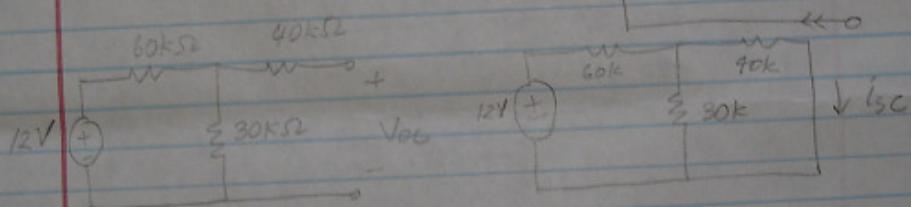
$$V_{oc} = \frac{30k}{30k+60k} (12V) = 4V$$
