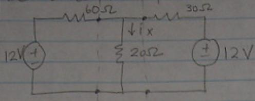
$$\frac{12V}{60\Omega} = 0.2A \quad \text{and} \quad \frac{12V}{30\Omega} = 0.4A$$
