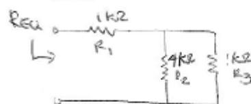
$$\begin{aligned} R_{eq} &= \left( \frac{1}{1} + \frac{1}{4} \right)^{-1} \\ &= \frac{4}{5} k\Omega \\ R_{eq} &= 1 + \frac{4}{5} \\ &= \frac{9}{5} k\Omega \end{aligned}$$
