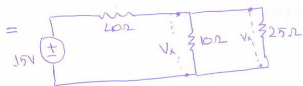
Resistance 10Ω and 25Ω are parallel so the potential difference
