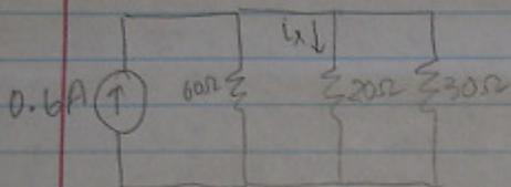
Since we need to find  $i_x$ , we leave the 20Ω resistor as it is and combine the other two resistors 60Ω and 30Ω ( $60\Omega \parallel 30\Omega$ )
