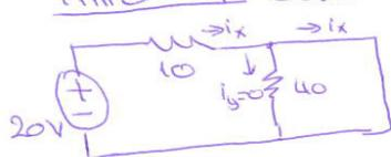
$$i_N = \frac{20V}{10\Omega} = 2A \text{ (by applying Ohm's Law)}$$
