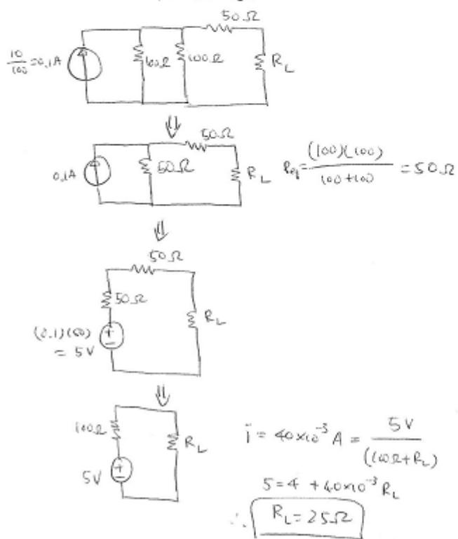
3.37) Find Thevenin equivalent circuit seen by  $R_L$  in figure. Find voltage across the load when  $R_L = 5\Omega, 10\Omega$  and  $50\Omega$ .
