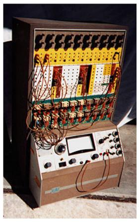
This is an analog computer from around 1963 It was used to solve nonlinear ODEs via analog circuitry
