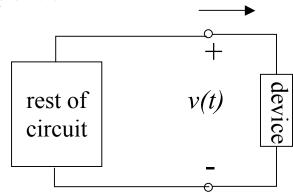
In the illustration the current into the device is the negative of that into the rest of the circuit
