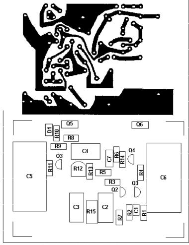
Figure 2. Amplifier Printed Circuit Board Layout
