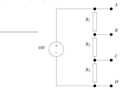
a) [2 marks] Show that if  $R_1 = R_3 = R\Omega$  and  $R_2 = 2R\Omega$  then  $v_A - v_B = v_C - v_D = 2.5V$  and  $v_B - v_C = 5V$ .
