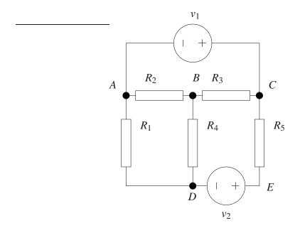
a) [2 marks] Transform the series connection of the voltage source  $v_2$  and the resistor  $R_5$  into an equivalent current source in parallel with a resistance and draw the resulting circuit.
