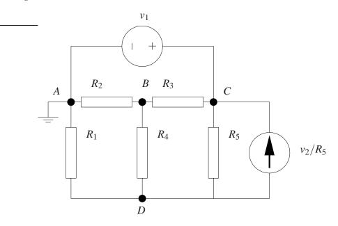
b) [3 marks] Formulate node-voltage equations for the resulting circuit. Remember to properly choose the ground node! Clearly state the unknowns and the equations to be solved.
