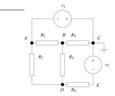
Now write the node-voltage equations by inspection. Because  $v_A = -v_1$  and  $v_E = -v_2$  are known we need only to write the current equations at nodes B and D. This results in
