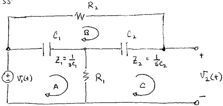
No initial energy  $\Rightarrow v_{c_1}(0) = v_{c_2}(0) = 0$
