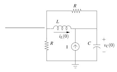
Transform to the s-domain using sources of current for initial conditions, as we will need to write node-voltage equations.
