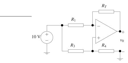
First recognize that the above circuit is a differential amplifier where
