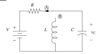
The first step is to determine  $v_C(0)$ . This is obtained by noticing that if the switch is on (A) for a long time then the current in C, and consequently in R, should be zero, therefore,  $v_C(0) = V$ .
