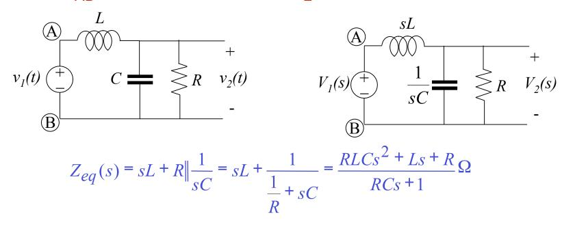
$$V_2(s) = \left[\frac{Z_1(s)}{Z_{eq}(s)}\right] V_1(s) = \left[\frac{R}{RLCs^2 + sL + R}\right] V_1(s)$$
