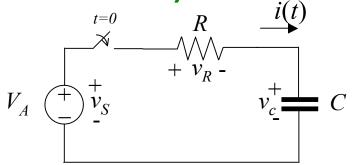
$$v_S(t) = V_A u(t), \quad v_R(t) = Ri(t), \quad i(t) = C \frac{dv_C(t)}{dt}$$
