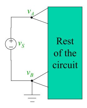
This removes the  $v_B$  variable – simpler analysis But can be done once per circuit
