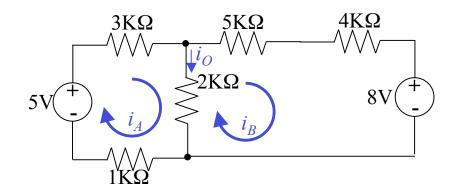
$$\begin{pmatrix} 6000 & -2000 \\ -2000 & 11000 \end{pmatrix} \begin{pmatrix} i_A \\ i_B \end{pmatrix} = \begin{pmatrix} 5 \\ -8 \end{pmatrix} \qquad i_A = 0.6290 \text{ mA}$$
