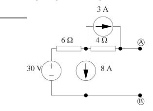
a) [4 marks] Determine the Thevenin equivalent as seen from terminals (A) and (B) using source transformations only.
