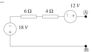
Combine the 12 V and the 18 V sources of voltage into a single 6 V source of voltage and associate the resistor to obtain the Thevenin equivalent circuit.
