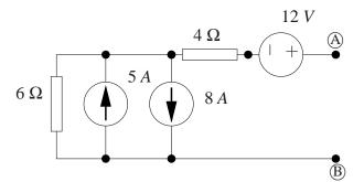
Combine the 5 A and the 8 A sources of current into a single 3 A source of current.
