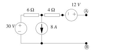
*Transform the* 30 V voltage source in series with the 6  $\Omega$  resistor.
