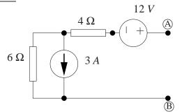
*Transform the* 3 A *current source in parallel with the* 6  $\Omega$  *resistor.*
