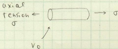
$$\begin{aligned} l &= 25 \text{ mm} \\ r &= 2.5 \text{ mm} \\ P_s &= 0.50 \\ \sigma &= 120 \text{ MPa} \end{aligned}$$
