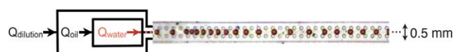
Fig. 1 Design of the microfluidic device. The flow-focusing module is coupled to a dilution module to induce localized jams along the 1D droplet stream. The colored water droplets are advected by a hexadecane phase. The flow focusing module is fed at the imposed flow rates: Q_{\text{water}} and Q_{\text{oil}} . Q_{\text{dilution}} is the hexadecane flow rate in the dilution channel.
