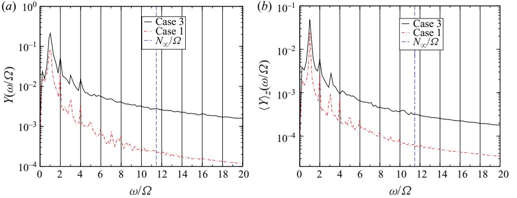
FIGURE 11. (Colour online) (a) Power spectra,  $Y$ , based on the time-series data of the baroclinic streamwise velocity at a location midway on the slope (point  $Q$  in the inset of figure 4) and inside the boundary layer for cases 1 and 3. The time series is taken over eight cycles and the spectra are averaged over the spanwise direction. The line average of the power spectra,  $\langle Y \rangle_z$ , is shown in (b). The dashed vertical line corresponds to the normalized buoyancy frequency.
