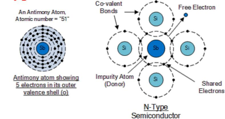
N-type Si has an extra electron for each dopant atom, This electron is mobile
