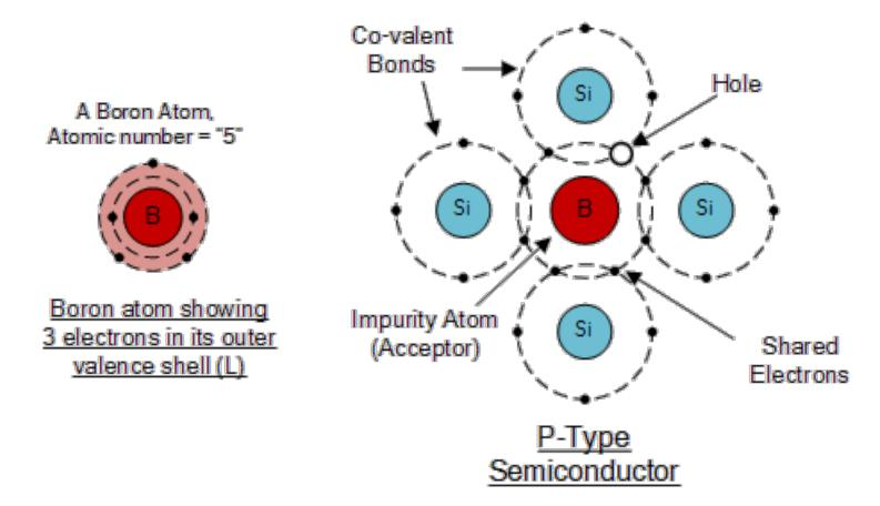
P-type Si has a "hole" (i.e a missing electron) that acts like A mobile positive charge
