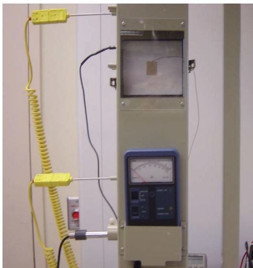
Figure 4: A close-up showing the heated plate and the velocity probe.
