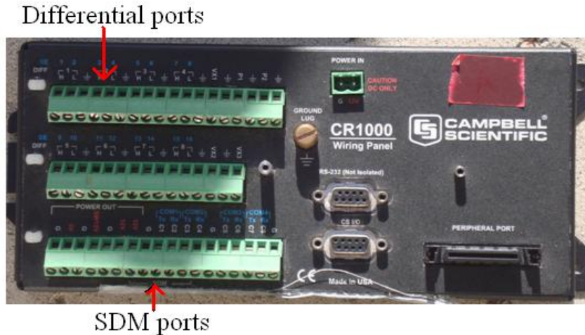
Figure 4. Differential (for net radiometer) and SDM ports (for CSAT) of the CR1000 datalogger.
