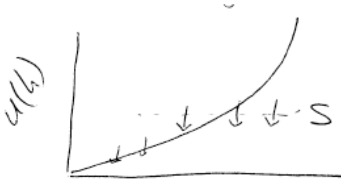
Figure 9.11: Sketch of the vertical flux S of horizontal kinetic energy
